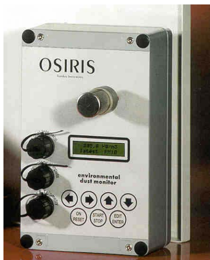
Photograph 1: The Turnkey Osiris Unit
